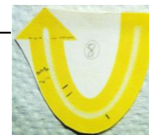
Sample volume optimization for determining ideal channel length
