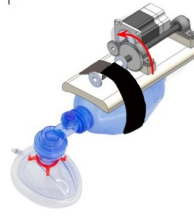
Figure 2: 3D rendered SolidWorks assembly of pusher plate compression mechanism. Red arrow indicates rotation of gear/shaft to wind compressive strap (black/gray) around spool (white).
