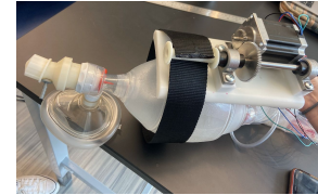
Figure 4: Physical construction of pusher plate assembly. Pictured on top of Ambu adult BVM.
