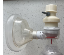
Figure 5: 3D Printed PEEP valve pressure sensing attachment. Shown attached to Ambu BVM PEEP valve.
