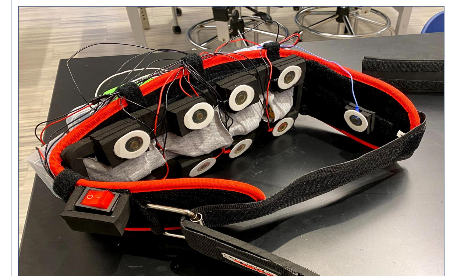
Figure 2: MSRD internal surface. Four pairs of EMG electrodes surrounding the vibrational motors.
